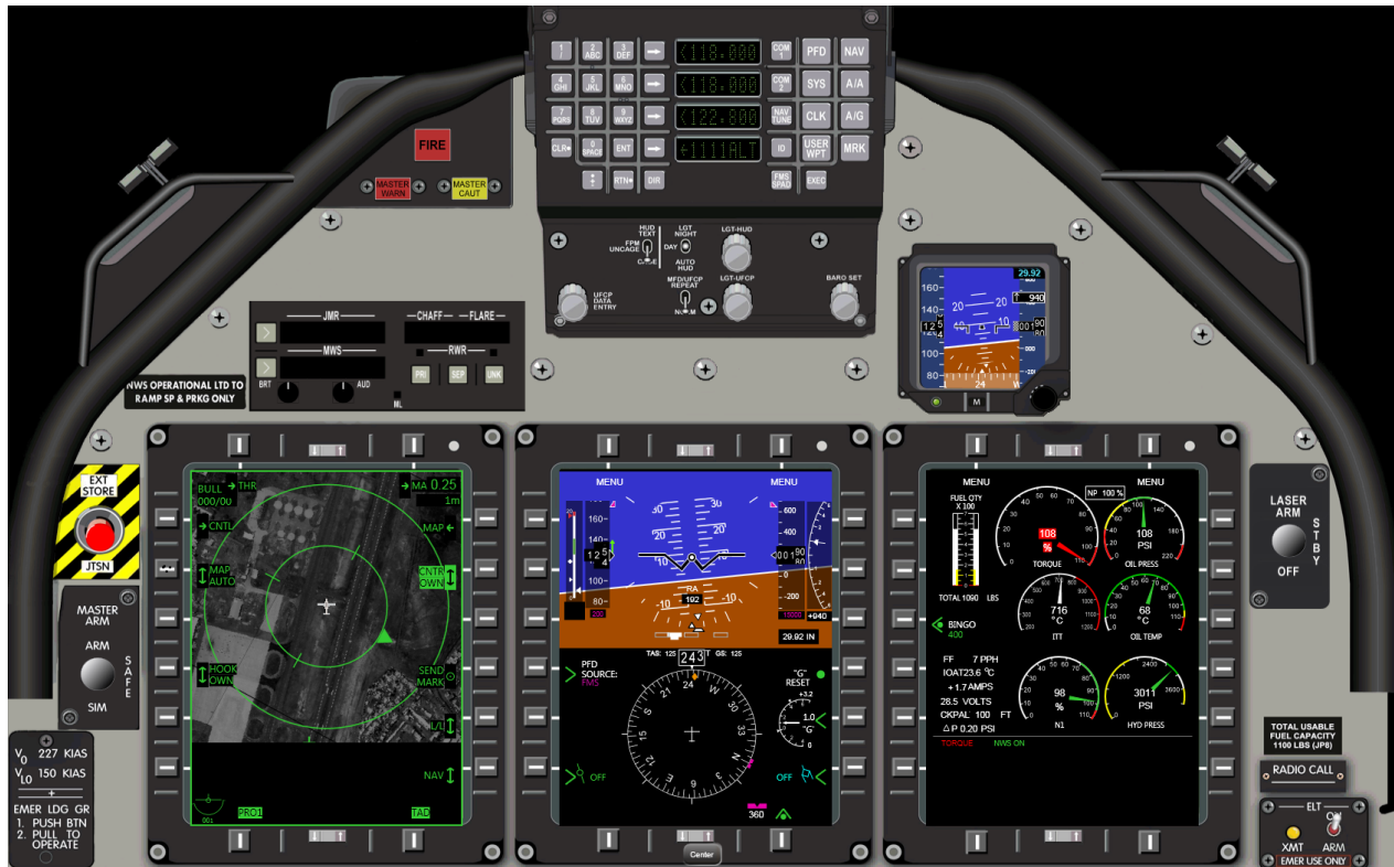
Figure 1. AT-6 Desktop Trainer with Moving Map, PFD, and EICAS displays (left to right)
